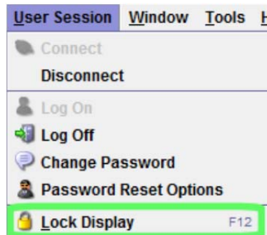
The Lock Display action may be performed by pressing F12 on the keyboard
